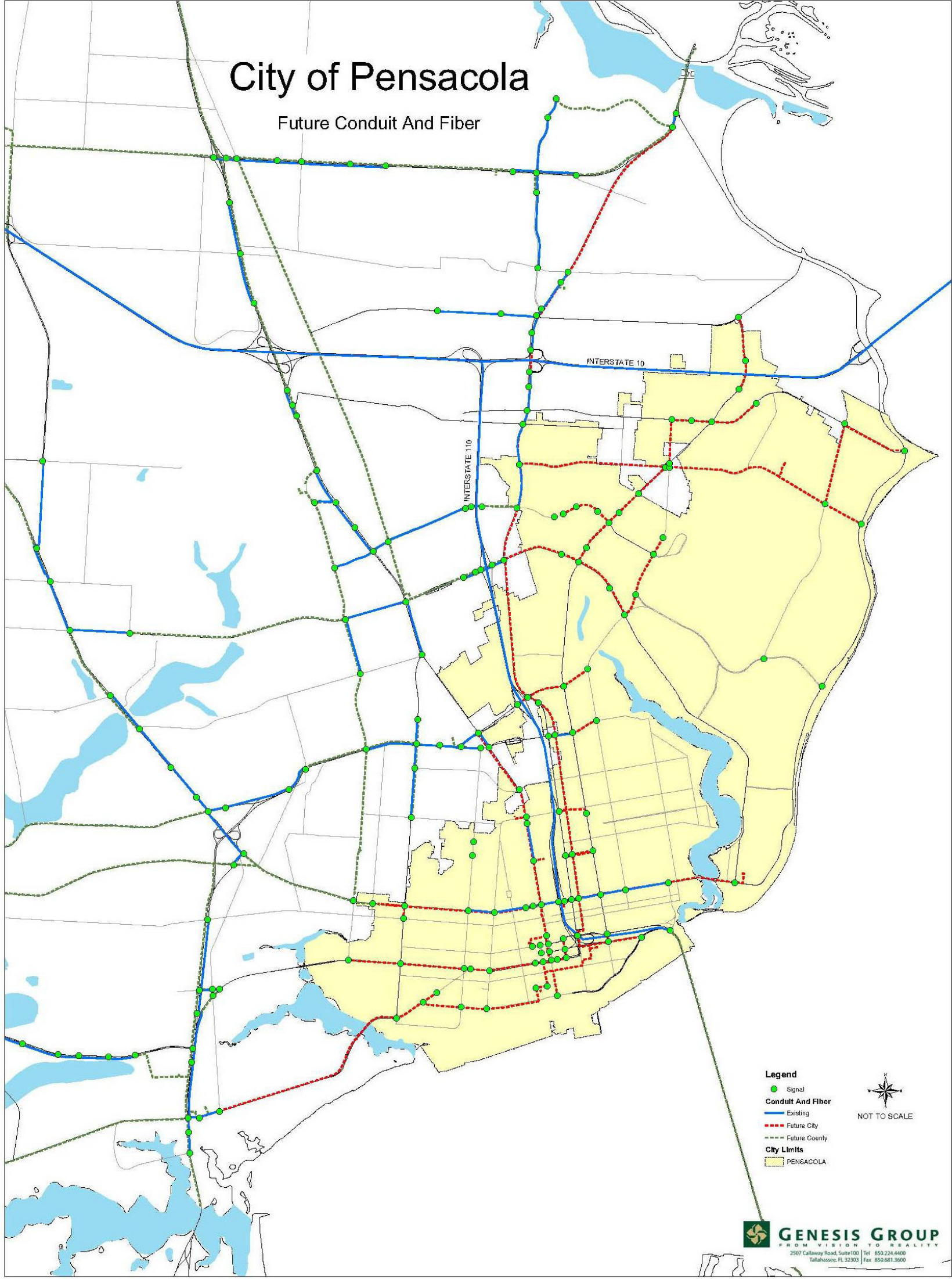
Figure 3.1.1.5 – Existing signalized intersections, existing and future fiber optic cable in the City of Pensacola, Florida
